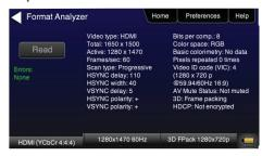
HDMI Source Audio Test – Run an audio test on an HDMI source device or A/V receiver to verify audio headers, audio infoframe and channel status bits.
