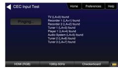
HDMI Source and Repeater Video Test – Test an HDMI source device directly or through a repeater. Verify timing, AVI Infoframes and HDCP authentication for standard video, deep color and 3D.
