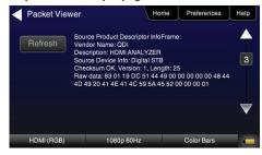
Testing Source's Response to an EDID – Provision 780's HDMI Input port with EDID from any display. Verify source responds properly to EDID. Load EDID from multiple stored EDIDs.
