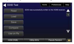
EDID Sink Testing – Run an EDID functional test on an HDMI HDTV and/or an A/V receiver to verify EDID checksum, header, and HDMI video and audio support. View entire EDID contents. Run portions of the EDID compliance test
